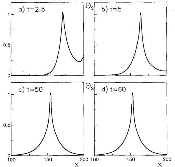
FIG. 5. The dynamics of temperature distribution in the superconductor,  $\theta_s$ , in the case of a pair of resistive domains. The parameters are  $\lambda=20$ ,  $\tau_m=3$ ,  $i=0.5$ .
