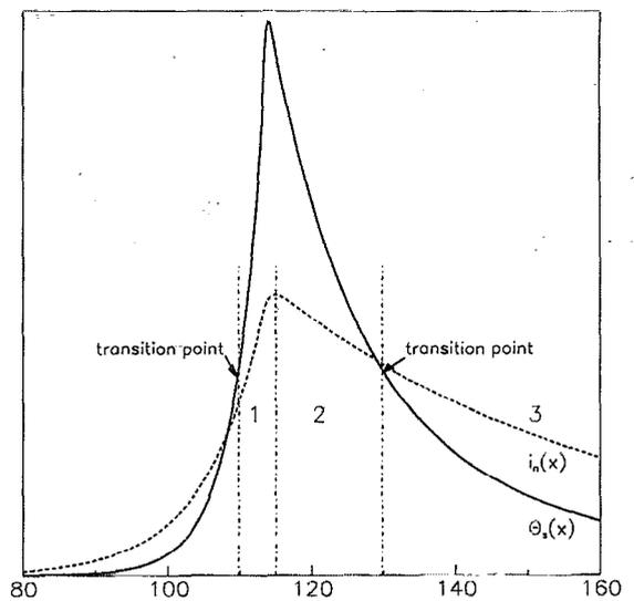
FIG. 9. Temperature distribution in the superconductor,  $\theta_s(x)$ , (solid line) and current-density distribution in the stabilizer,  $i_n(x)$ , (dashed line) in a propagating normal domain.
