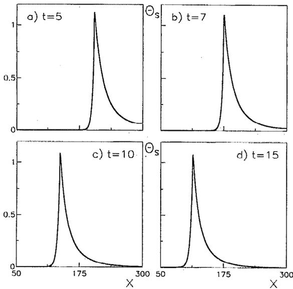
FIG. 7. The dynamics of temperature distribution in the superconductor,  $\theta_s$ , in the case of propagating normal domains. The parameters are  $\lambda=20$ ,  $\tau_m=5$ ,  $i=0.6$ .
