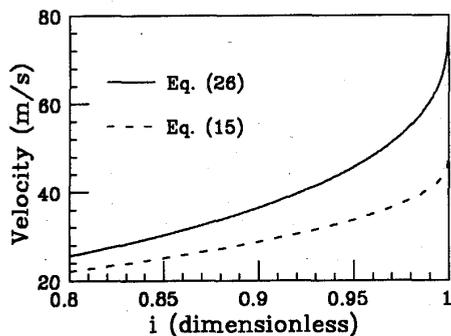
Figure 3: The dependence of the quench propagation velocity  $v$  on the dimensionless current  $i$ .
