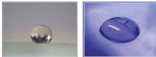
**Fig. 1** Left: A drop of water on a surface with low polarity (hydrophobic), such as Teflon or greased baking paper. The drop draws itself into a ball and there is little wetting. Photograph: Vincent Kwong, UBC. Right: A drop of water on a surface of higher polarity. The drop flattens out and high wetting occurs. Photograph: Betty Winter.
