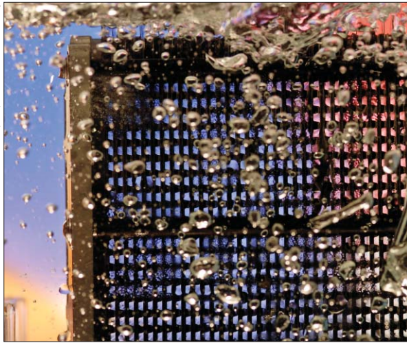
Bubbling away A fuel cell generates electricity by reacting oxygen, hydrogen ions and electrons (artist's impression, left). The hydrogen ions generated at the anode are swept through a membrane to the cathode. The membrane is often made from a polymer called Nafion, which has a Teflon skeleton with negatively charged groups of sulphur trioxide attached to it. This membrane is impermeable to electrons generated at the anode, which are routed to the cathode via an external circuit that is powered by the cell.
