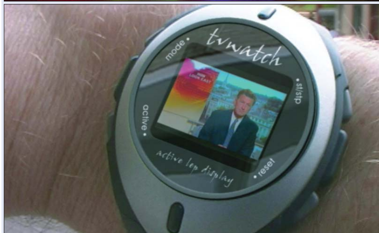
An example of coloured light emitted from specific polymers in response to being illuminated by white light, with no source of electricity (top). Each polymer has its own characteristic colour. A small television screen made of PLED mounted on a watch (bottom).
