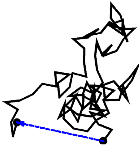
Figure 1. Example of a random Brownian walk of 100 steps in the plane, drawn from a computer simulation. The blue arrow connects the initial point to the final point. Note how short the arrow is relative to the length of the entire path. If the length of a single step is a , the entire path length is 100a . In contrast to this, if we were to draw many processes such as that of the figure and work out the average arrow length, we would find a length of only 10a .
