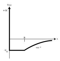
Fig. 14. A typical surface potential felt by a monomer as a function of the distance x from an adsorbing surface. First the surface is impenetrable. Then, the attraction is of strength  $V_0$  and range B. For separations larger than B, typically a long-ranged tail exists and is modelled by  $-wx^{-\tau}$ .
