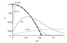
Fig. 28. Results for the density profile (normalized to unity) of a strongly compressed brush, as obtained within mean-field theory. As the compression increases, described by the stretching parameter  $\beta$ , which varies from 0.1 (dots) to 1 (dash-dots), 10 (dashes), and 100 (solid line), the density profile approaches the parabolic profile (shown as a thick, dashed line) obtained within a classical-path analysis (adapted from Ref. [290]).
