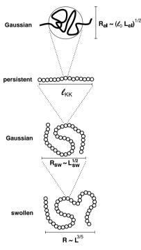
Fig. 7. Schematic view of the four scaling ranges in the Gaussian-persistent regime. On spatial scales smaller than  $R_{\rm el}$  the chain behavior is Gaussian; on length scales larger than  $R_{\rm el}$  but smaller than  $\ell_{\rm KK}$  the Gaussian blobs are aligned linearly. On larger length scales the chain is isotropically swollen with an exponent  $\nu = 1/2$ , and on even larger length scales self-avoidance effects become important and the exponent changes to  $\nu = 3/5$ .
