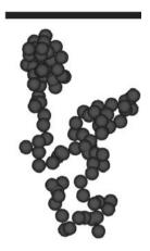
Fig. 3. Snapshot of a Monte-Carlo simulation of a neutral freely jointed chain (FJC) consisting of N = 100 monomers with a diameter corresponding to the Kuhn length a. The theoretical end-to-end radius, R = 10a, is indicated by the upper horizontal bar.
