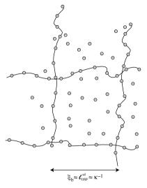
Fig. 9. Schematic view of the PE chain structure in the semi-dilute concentration range. The mesh size  $\xi_b$  is about equal to the persistence length  $\ell_{OSE}^{sd}$  and to the screening length  $\kappa^{-1}$  (if no salt is added to the system).
