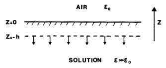
FIG. 1. A flat interface at z = 0 separates air (dielectric constant  $\epsilon_0$ ) from an aqueous solution ( $\epsilon \ge \epsilon_0$ ). Dipoles are confined to the plane z = -h.
